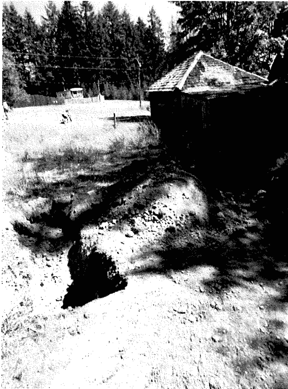
Soil test pit at site showing clay, stones and cobbles, soils that are mapped as 5 PA (stony and arid)
