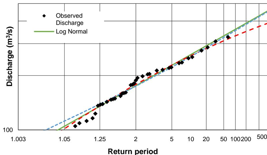
**Figure 5-5: Frequency analysis of annual maximum discharges at outlet of Cowichan Lake (Gauge 08HA002).**
