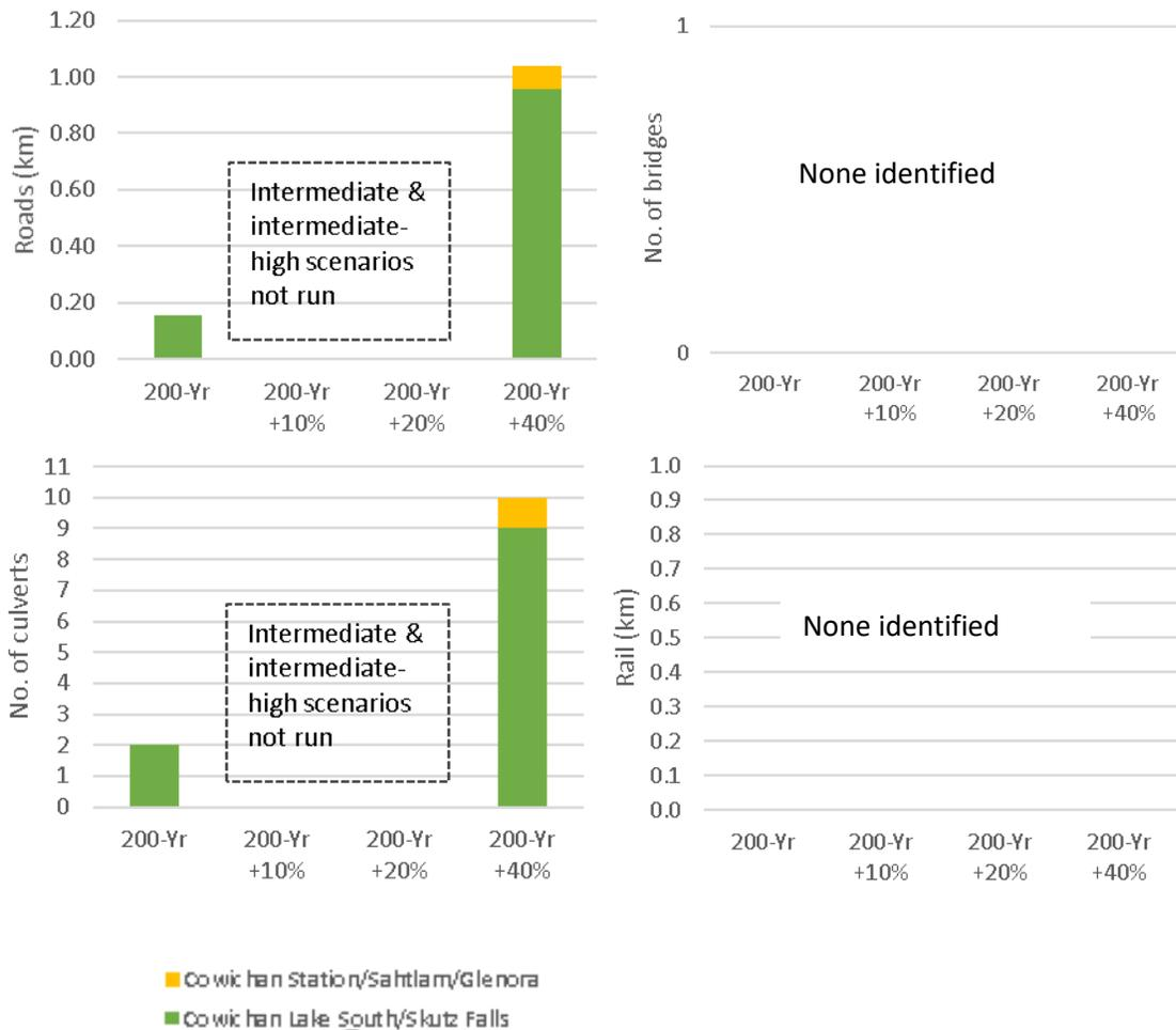
**Figure 7-11: Local infrastructure impacts – quantified flood exposures (transportation infrastructure).**
