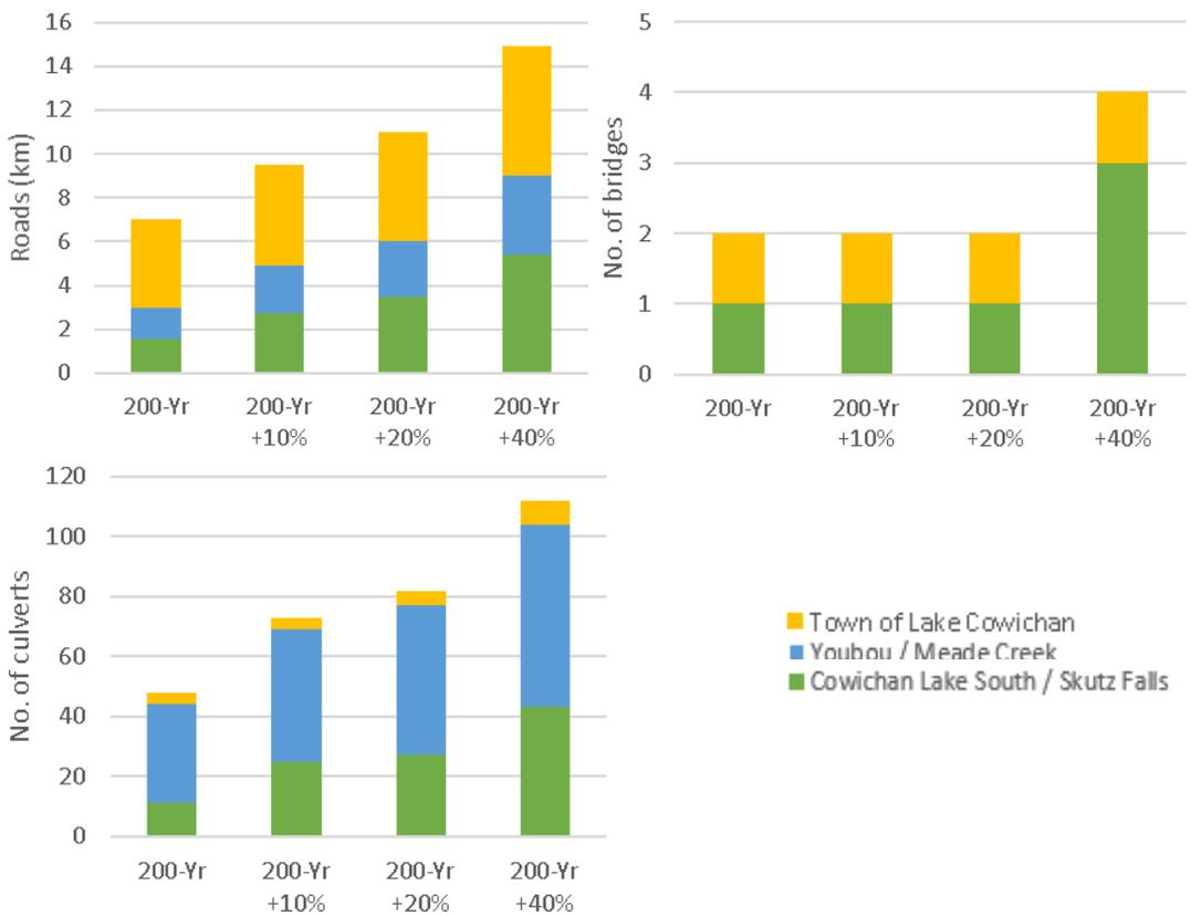
Figure 5-20: Local infrastructure impacts – quantified flood exposures (transportation infrastructure).
