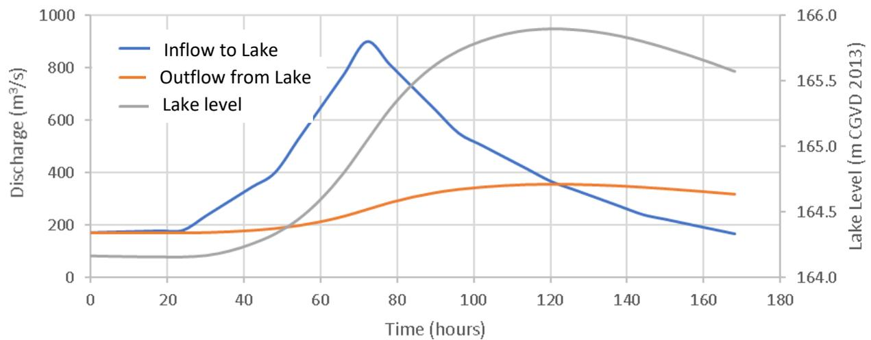
**Figure 5-8: Computed lake level and river outflows during the projected 200-year flood event.**
