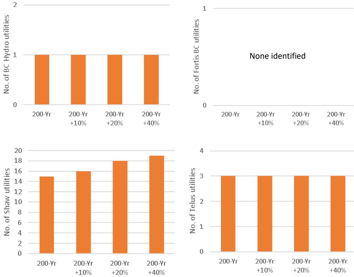
**Figure 6-8: Local infrastructure impacts – quantified flood exposures (Shaw, Hydro, Telus).**
