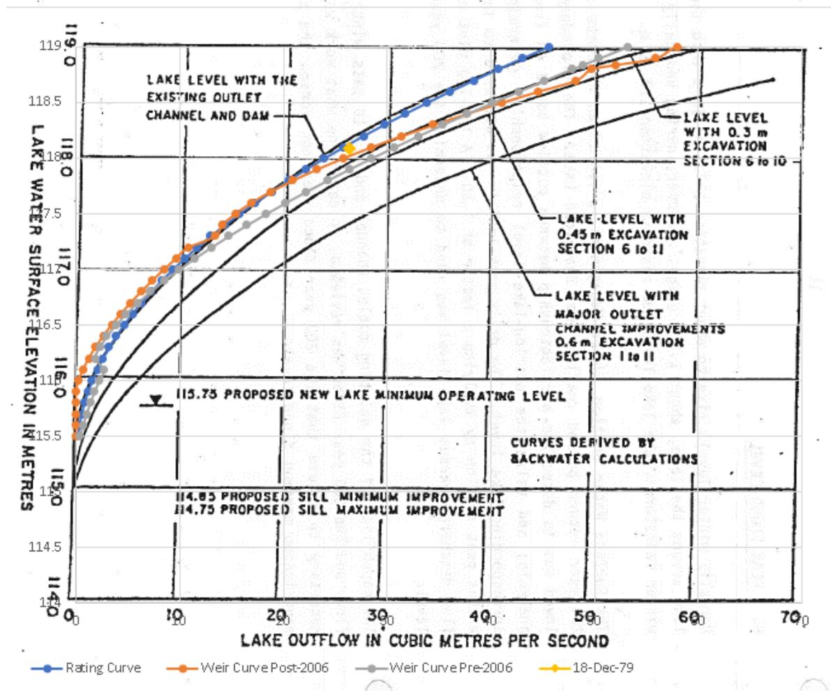
**Figure 6-3: Discharge elevation curve by Talbot (1985) fitted with a rating curve and overlain with Weir equations for Pre- and Post-2006. Figure elevations shown in CGVD1928 HT97.**
