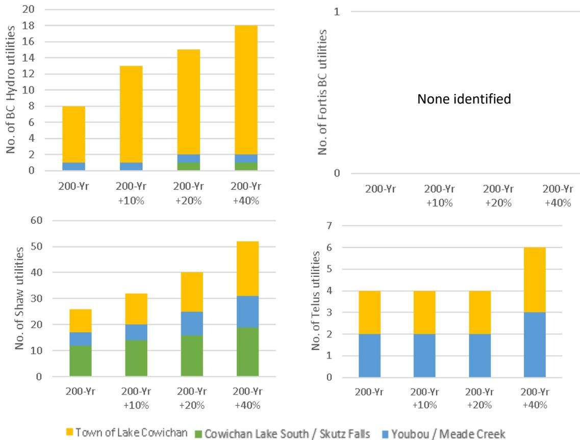
Figure 5-18: Local infrastructure impacts – quantified flood exposures (Shaw, Hydro, Telus).
