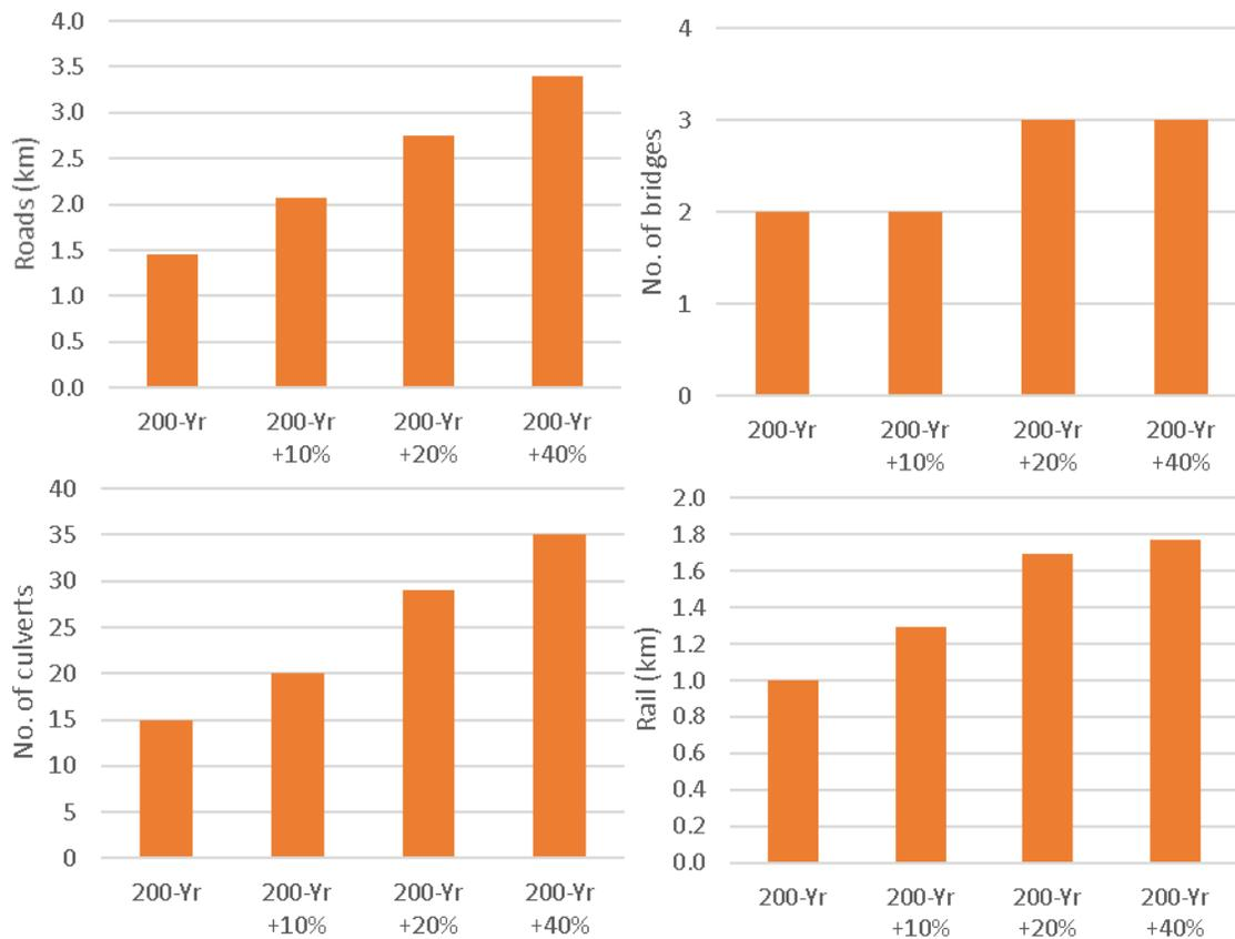
**Figure 6-10: Local infrastructure impacts – quantified flood exposures (transportation infrastructure).**
