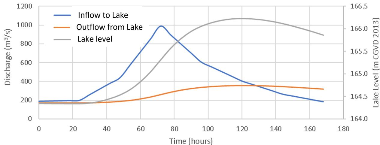
**Figure 5-9: Computed lake level and river outflows during the projected 200-year flood event. The estimated 200-year lake inflow hydrograph was increased by 10% to account for a moderate increase due to climate change.**
