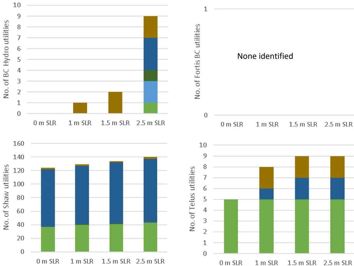
**Figure 10-11: Local infrastructure impacts – quantified flood exposures (Shaw, Hydro, Telus).**
