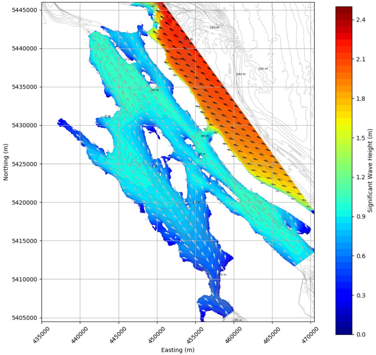
**Figure 10-3: Significant wave heights calculated for Georgia Strait (SWAN model nested grid) for a south-easterly 10-year wind event.**
