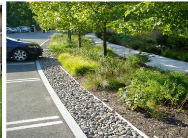
Image 33: Pervious, landscaped surfaces and light reflective surfaces minimize heat absorption.
