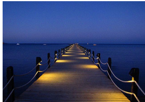
Image 12: Full cut-off luminaires limit light pollution to reduce impact on marine life.
