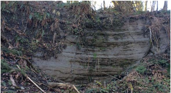
Photo 1: Varved silt and fine sand exposed in a landslide on 5451 Allenby Road.
