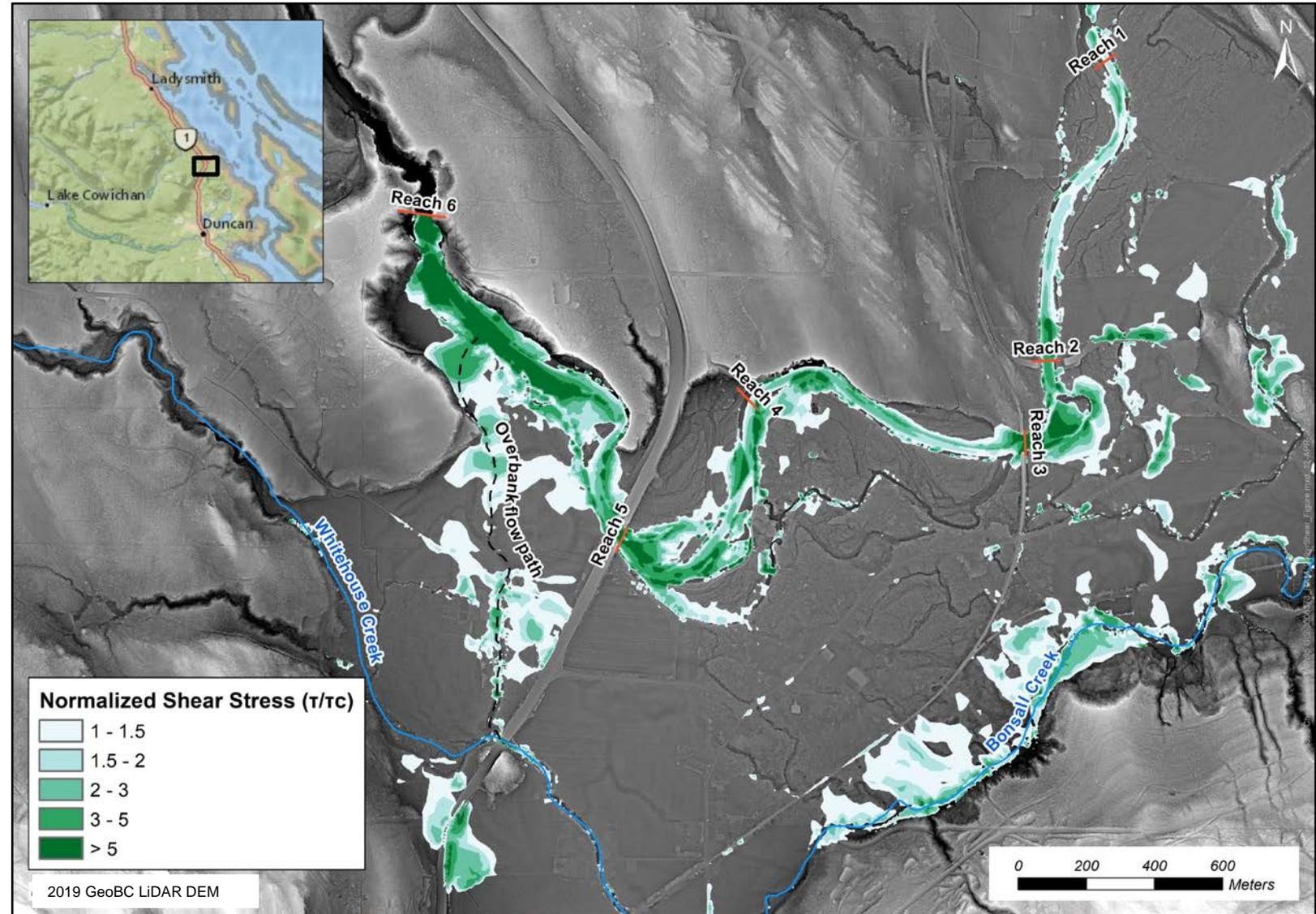
▲ The normalized shear stress produced during a 2D HEC-RAS hydraulic model simulation of a 0.5% AEP flood with a 20% increase in discharge to account for climate change. Normalized shear stress is calculated as the ratio of shear stress ( $\tau$ ) to critical shear stress ( $\tau_c$ ) for sediment entrainment. Here, a critical shear stress of 25 Pa was used, an approximate threshold for mobility of coarse gravels (USGS, 2013).
