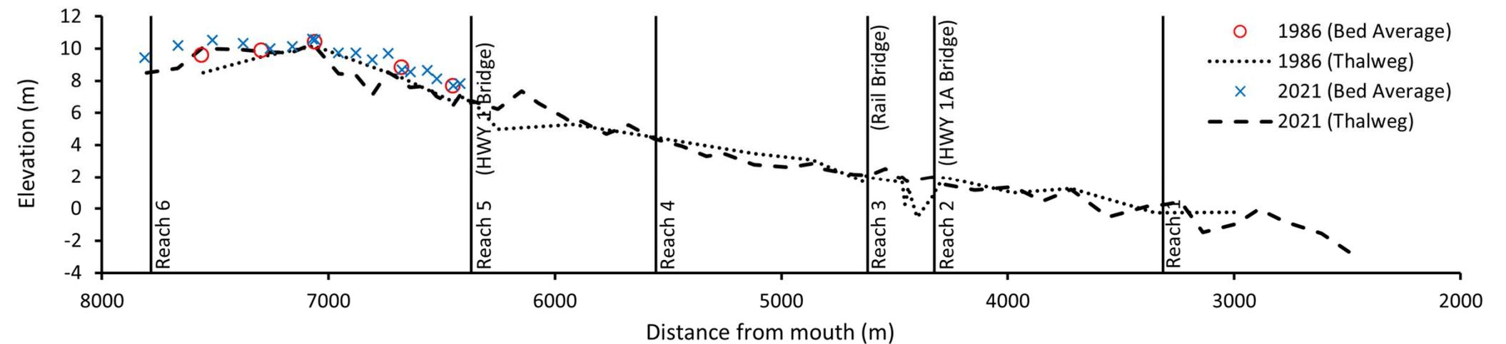
▲ Plot showing average bed elevation and thalweg elevation data from 1986 and 2021 survey data. Average bed elevation represents the average elevation at each cross section, including the deepest parts of the channel, top of exposed channel bars and all points in between.
