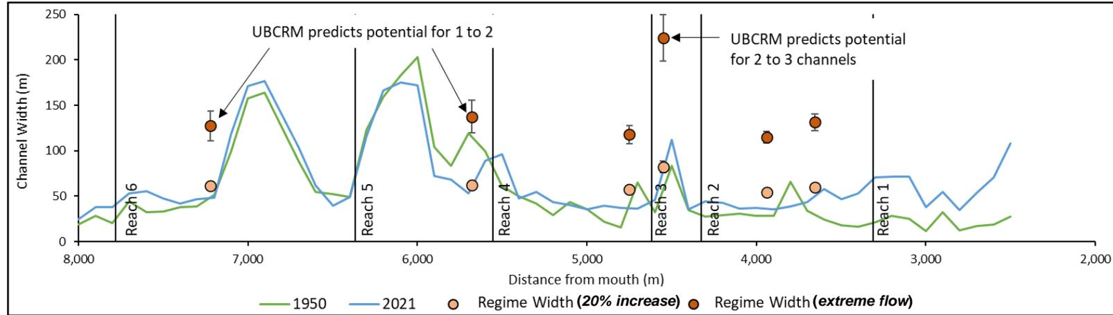
The UBCRM predicts that the river will widen by 6 to 11 m in response to an increase of 20% in the channel forming discharge ( $Q_{reference}$ ). This falls within the projected erosion hazard area buffers, as depicted in the geomorphic hazard map (Page 44).
