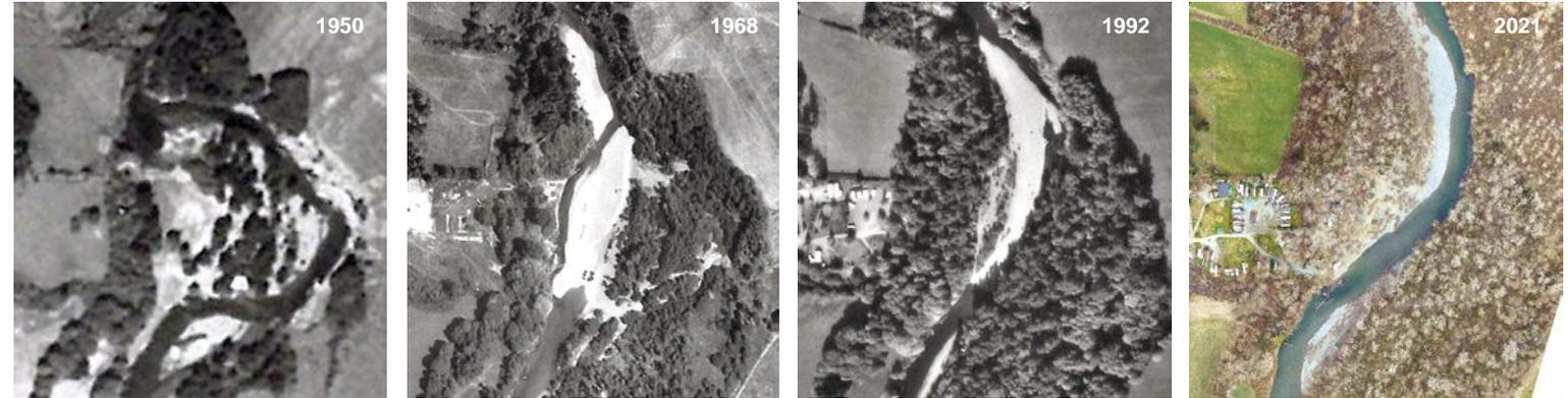
▲ A channel avulsion occurred between 1950 and 1968. Since then, the gravel bar has become increasingly stable as vegetation has established on the bar interior. The bar and meander bend have migrated downstream since 1992 as sediment is eroded from the bar head area and deposition occurs on the bar tail.
