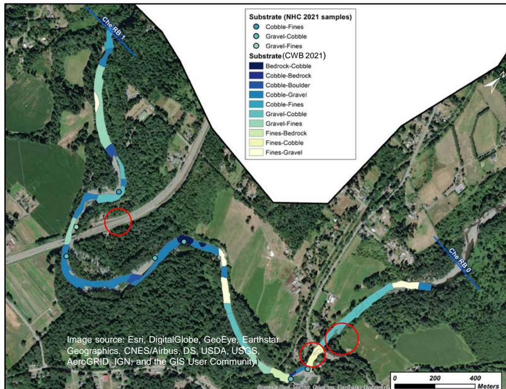
▲ Stream substrate classification. Red circles highlight localized sediment fining upstream of bridges.
