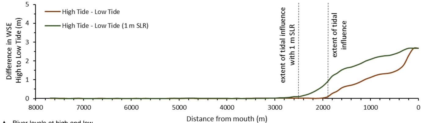
▲ River levels at high and low tide based on the mean annual tide and bankfull flow conditions ( $Q_{reference}$ ). WSE = water surface elevation.
