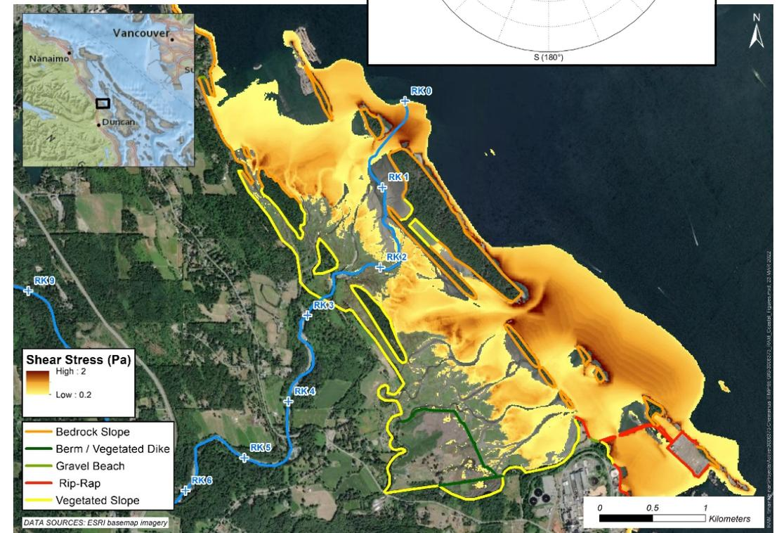
▲ Wave shear stress from SWaN model simulations of northerly (left panel) and east-southeasterly (right panel) annual wind events. The northerly wind event produces higher magnitudes of shear stress near the main channel of the Chemainus River, while the east-southeasterly event produces shear stress across a wider area of the estuary. The bedrock and rip-rap shorelines are likely to be resistant to erosion, while the gravel beaches and vegetated slopes are more likely to erode at a higher rate.
