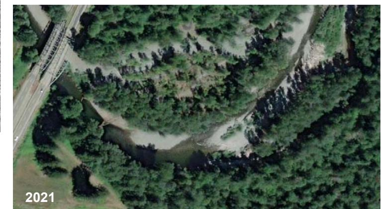
▼ Photo 5.12 Fine to medium gravel and sand is transported through a back-channel along the inside of the point bar. The channel is about 2.5 m wide and incised approximately 0.3 m into the floodplain.
