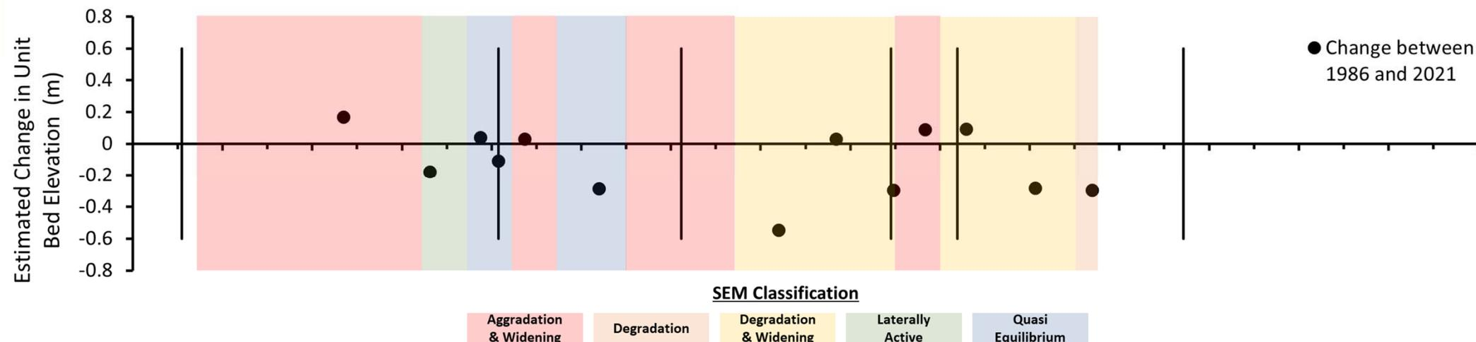
SEM classes reflect the geomorphic condition of the channel. The SEM classes consider the cyclical nature of channel evolution, whereby the channel transitions between periods of aggradation, degradation and quasi-equilibrium.
