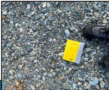
▶ Example of the fine to medium gravels deposited on the bar surface at the pebble count location.
