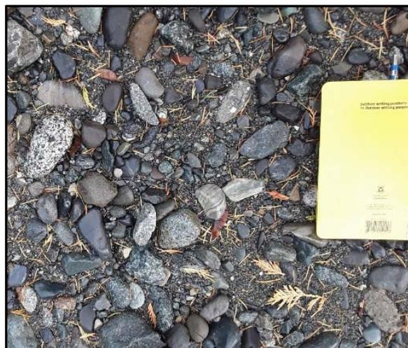
▲ Pebble count taken at RK 6.45, just upstream of the Highway 1 bridge. D<sub>90</sub> refers to the sediment grain size diameter that is not exceeded 90% of the time in the sample dataset.
