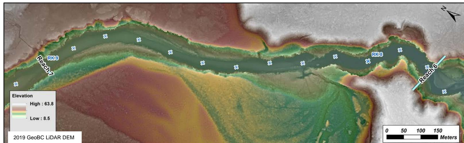
**Note:** RK refers to the River Kilometer distance measured along the channel thalweg, upstream of the approximate seaward extents of the estuary (northeast of the northern Willy Island passage). Each 100 m channel distance is marked with an 'X' and every RK is labelled.
