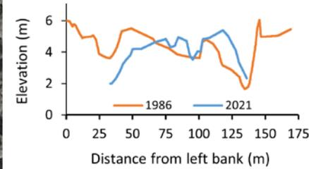
◀ Surveyed bed elevations at the mid-channel bar at RK 4.5. Between 1986 and 2021, the left channel deepened and widened. Accretion occurred along the right margin of the mid-channel bar and within the right channel.
