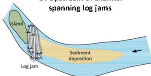
◀ The schematic at left (after NHC, 2015a) illustrates discrete locations where sediment conceptually is more prone to depositing along a stream channel.
