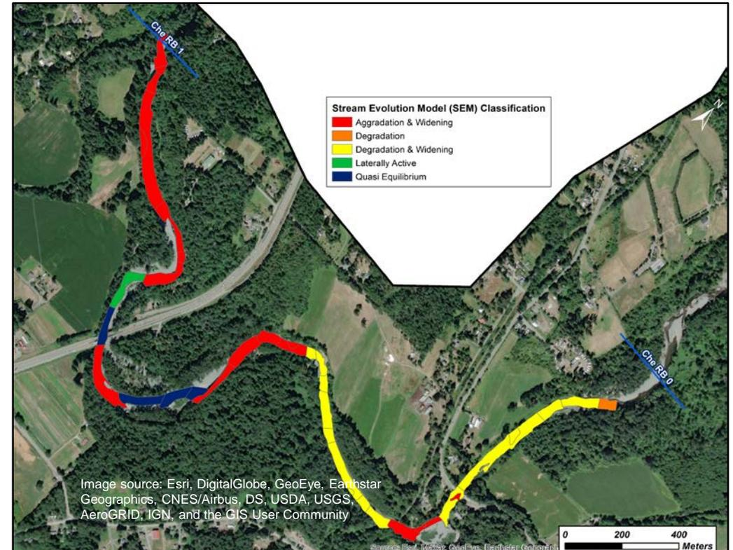
▲ Stream Evolution Model (SEM) classification of the channel's geomorphic condition.
