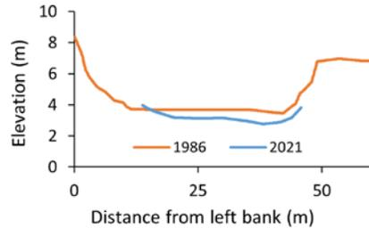
Plot showing scour at RM 5.1 between 1986 and 2021 based on repeat surveys.
