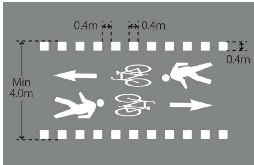
**Figure 5.5 Combined Crossing with Green Pavement Markings**
