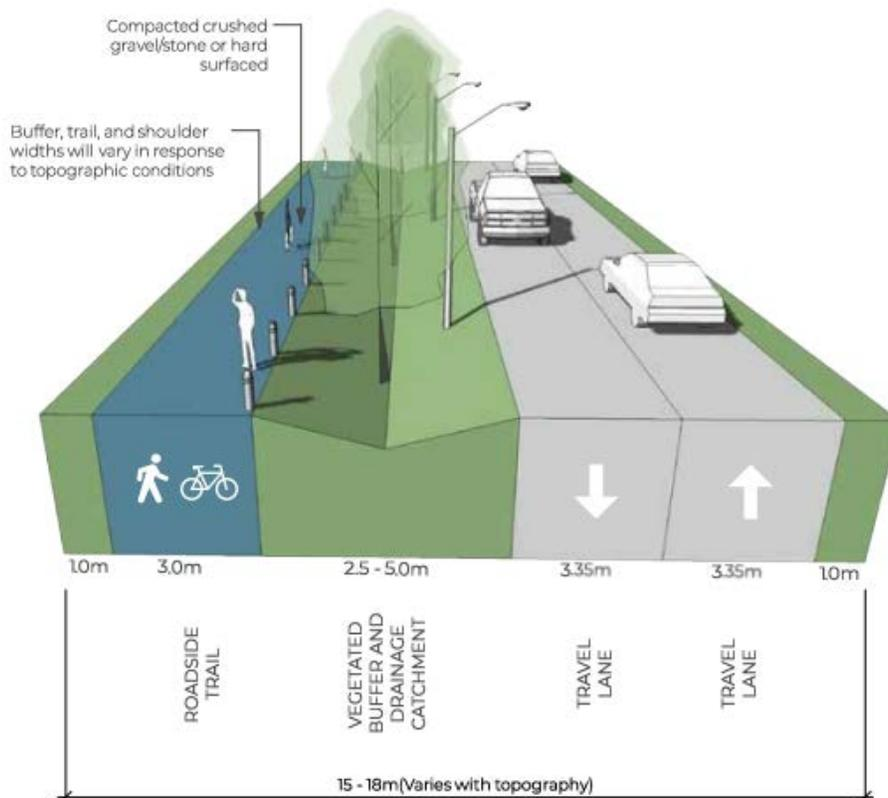
**Figure 5.3: Potential MUP Cross Section**
