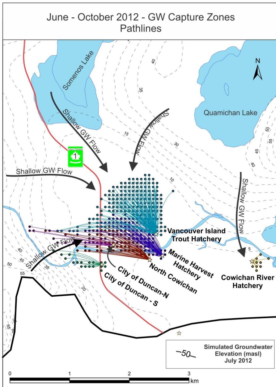
**Figure 3.13. Summer low flow season transient capture zone analysis results for the major GW extraction users within the lower valley. Shown are the particle pathlines within the shallow aquifer materials.**
