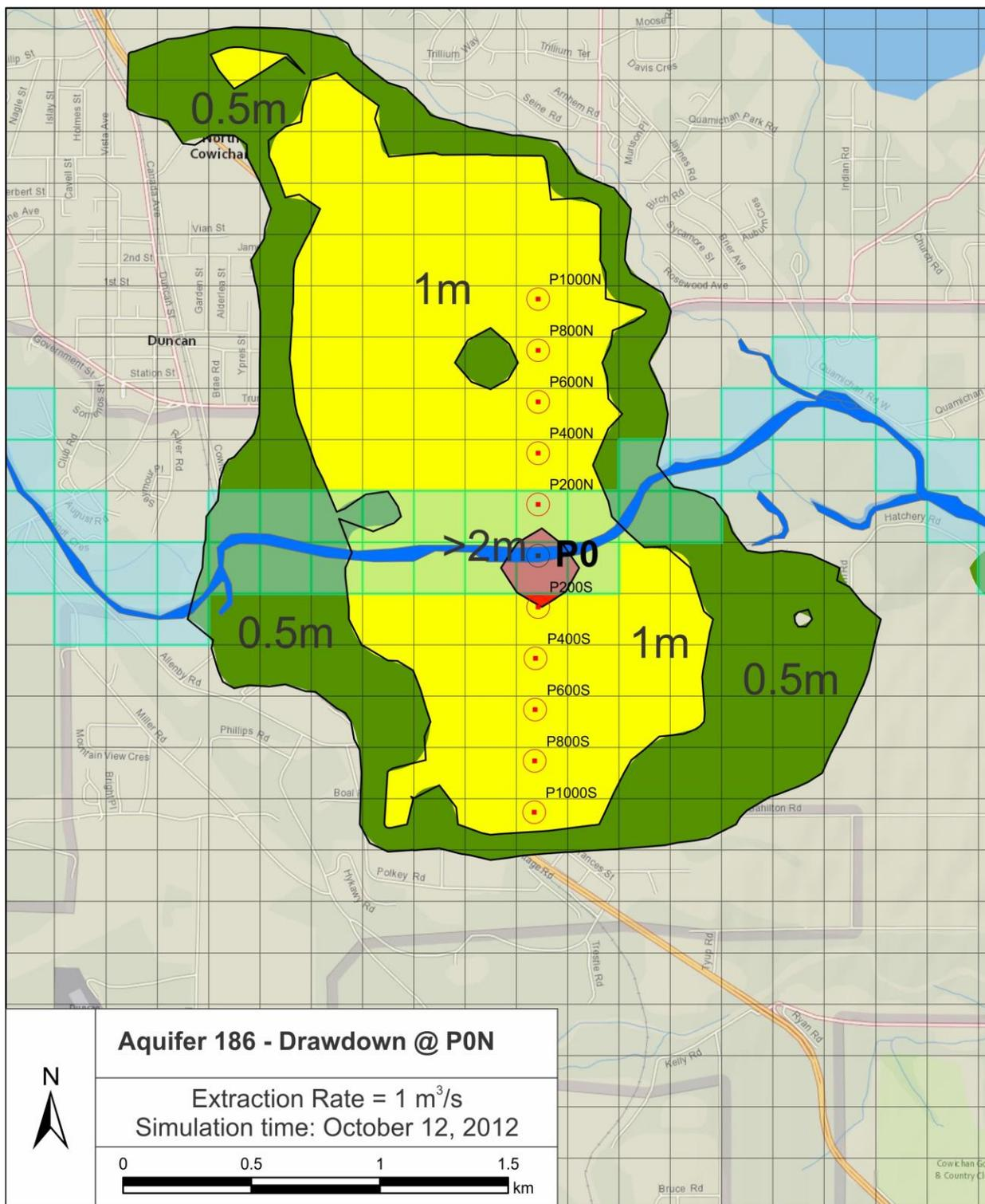
Figure 3.21. Drawdown during distance - sensitivity test. Pumping occurring at P0 location (1 m<sup>3</sup>/s).
