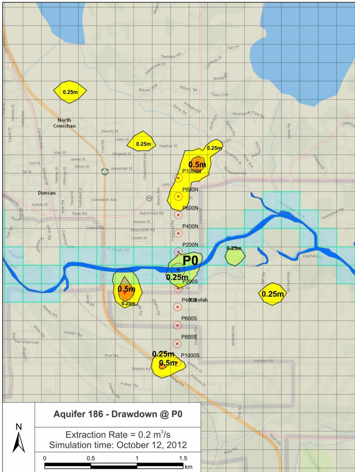
Figure 3.25. Drawdown during distance - sensitivity test. Pumping occurring at P0 location (0.2 m<sup>3</sup>/s).
