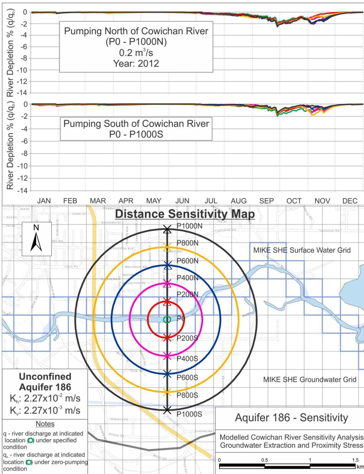
**Figure 3.24. Modelled Cowichan River distance - sensitivity assessment for Aquifer 186 (0.2 m<sup>3</sup>/s pumping rate).**
