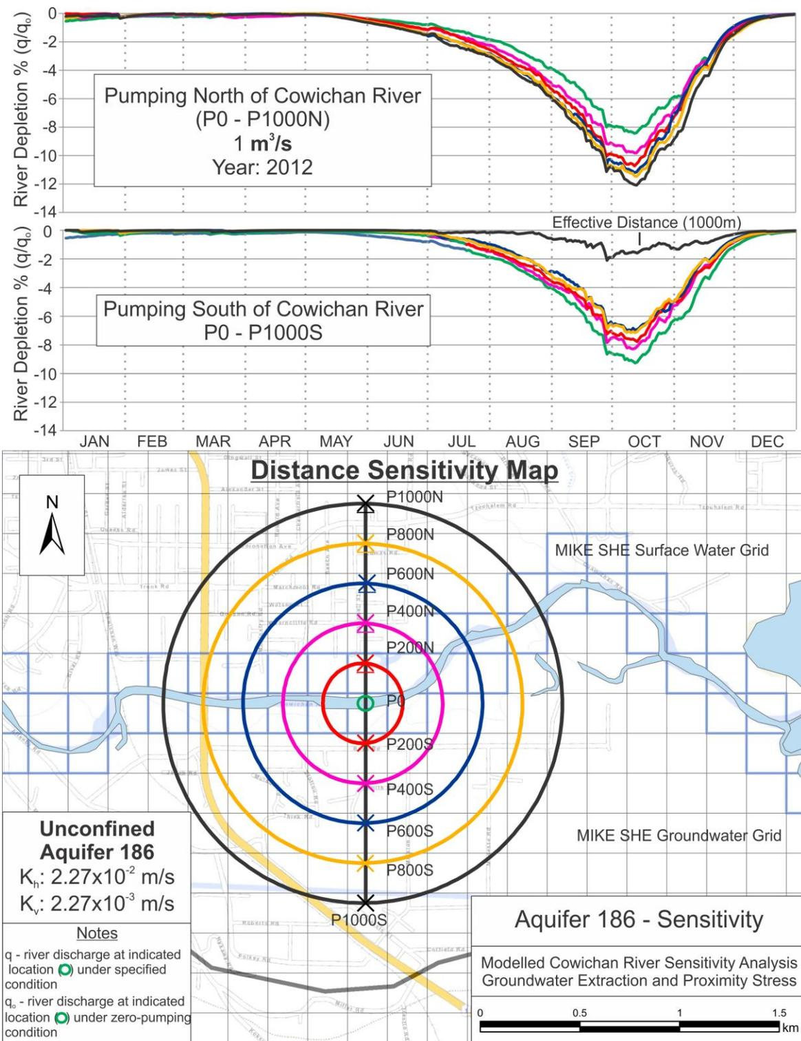
**Figure 3.20. Modelled Cowichan River distance - sensitivity assessment for Aquifer 186 ( $1 \text{ m}^3/\text{s}$  pumping rate).**
