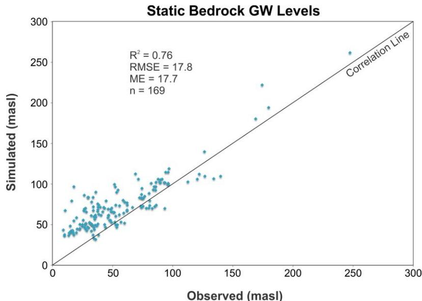
**Figure 3.2. Simulated mean annual (2007) bedrock GW elevations versus observed static GW elevations in bedrock from the BC WELLS database.**
