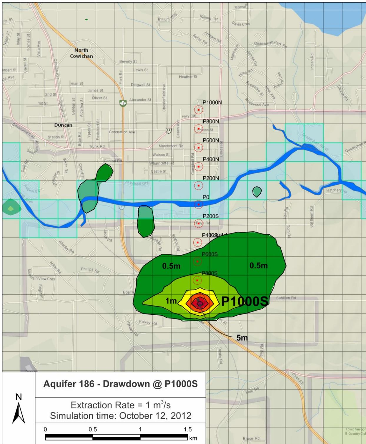
Figure 3.23. Drawdown during distance - sensitivity test. Pumping occurring at P1000S location (1 m<sup>3</sup>/s).
