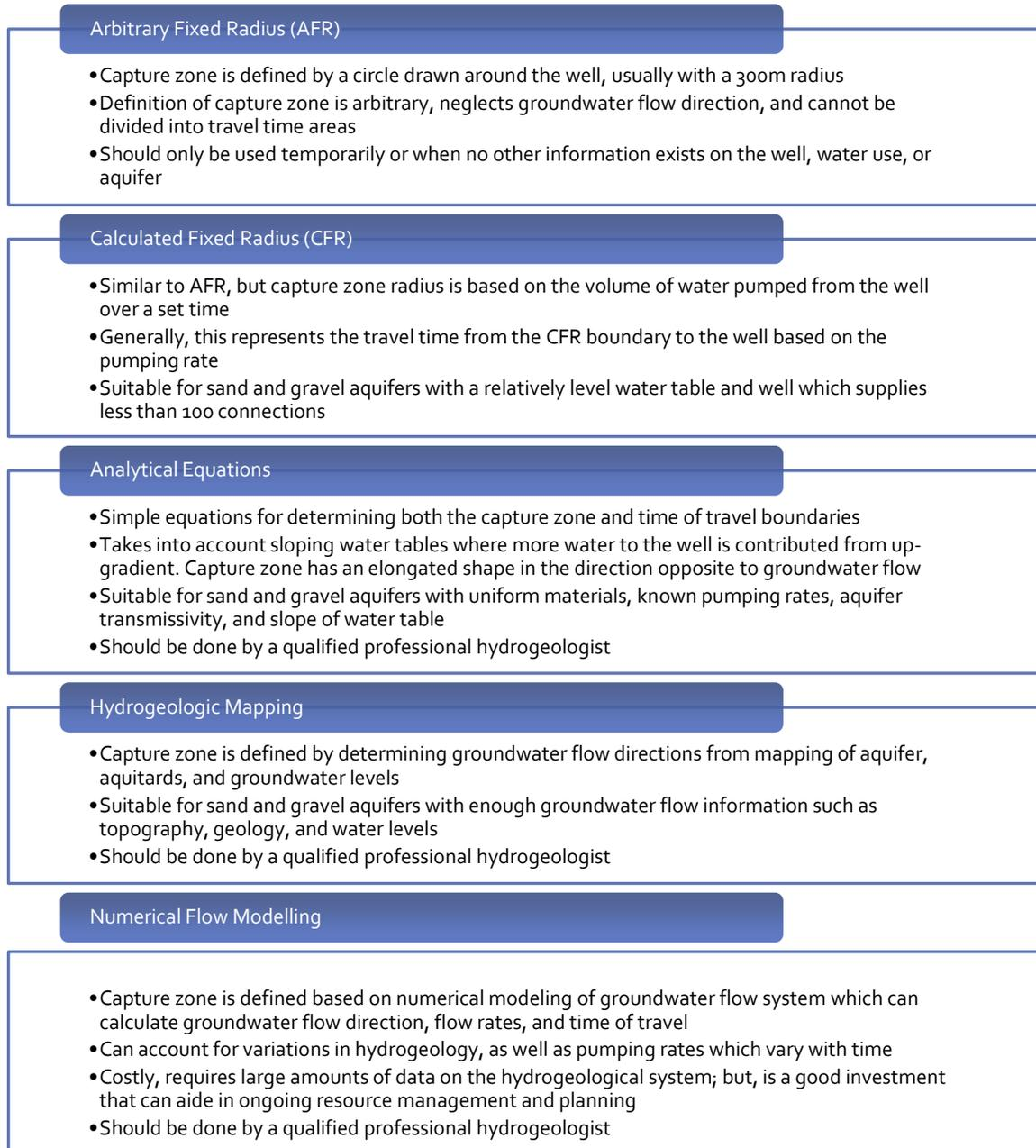
Figure 14: Well capture zone delineation according to the BC Protection Toolkit<sup>21</sup>.
