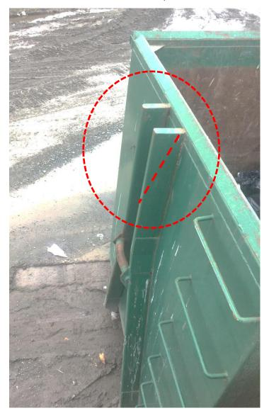
**Image #2:** Safety Chain Securement – The grade-70 grab hook must be attached to Container; no slots are to be cut in Containers.
