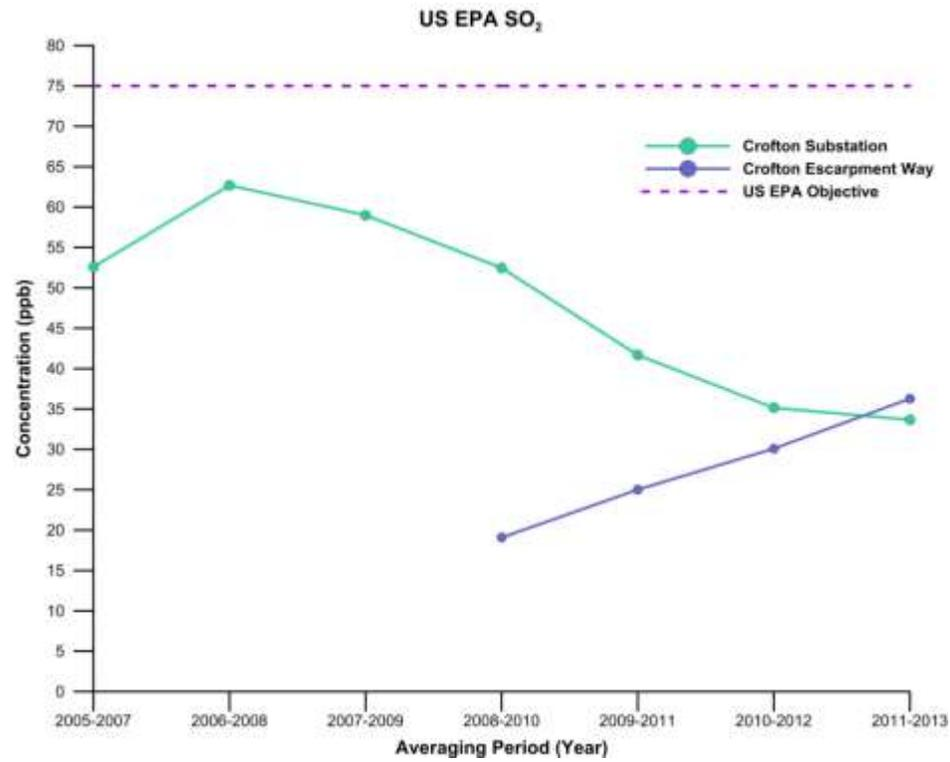
**Figure 8. 1-Hour Average SO<sub>2</sub> Results for the US EPA Supplemental Objective at the Crofton Substation and Crofton Escarpment Way Monitoring Stations**
