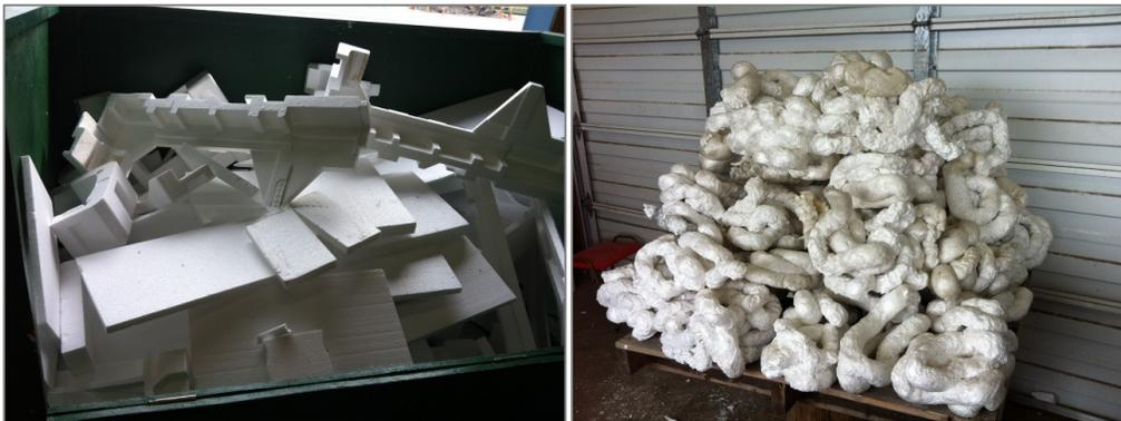
*Polystyrene foam before and after processing through the densifier*
