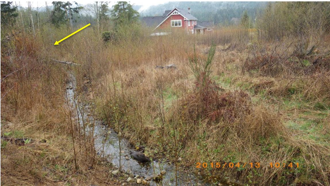
Figure 43. Looking south along the man-made stream that encircles the residential building. Note the stream flow in the stream channel that consists of a mix of flow from the wetland and surficial over land flow from the steep hillside lying to the east. Near surface ground water is also intercepted by the stream channel. The yellow arrow is the location of the image shown in Figure 44.
