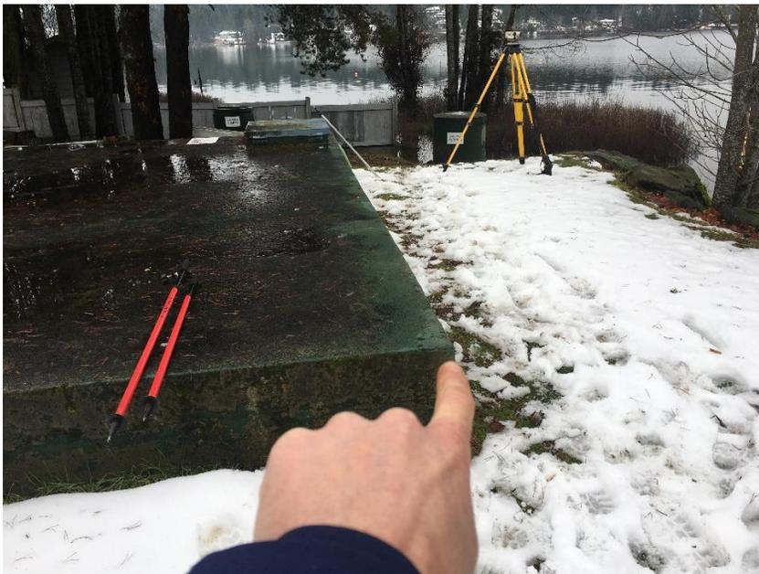
Photo 3: Benchmark NHC1111 (elevation= 119.483m), corner of concrete pad
