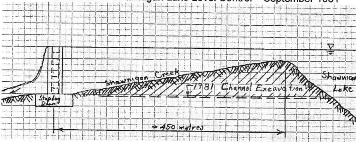
**Figure 6: Varying lake level control due to sediment accumulation and excavation carried out in 1981 by BC MoE (reproduced from Bryden and Barr, 2002)**
