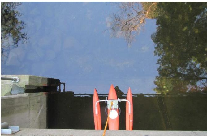
Photo 2: ADCP discharge measurement at Shawnigan Lake Weir
