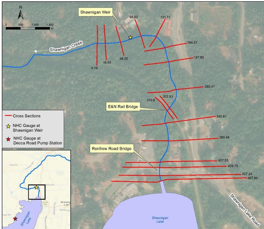
**Figure 2: Shawnigan Creek channel and floodplain cross sections**
