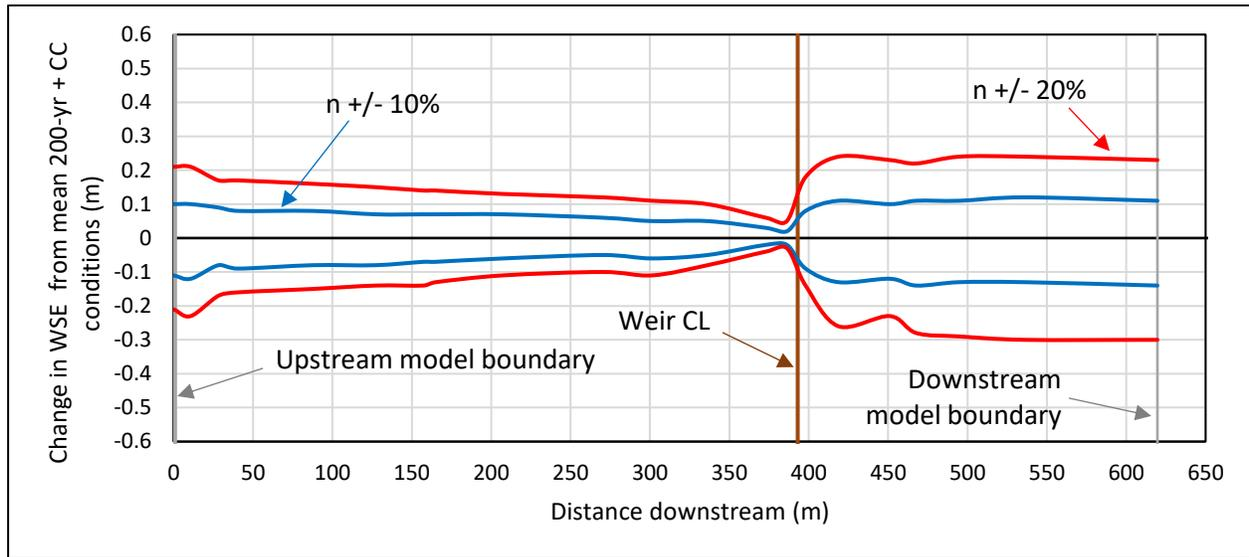
**Figure 21: Model sensitivity analysis results for change in Manning’s n for the closed Shawnigan Lake Weir scenario**
