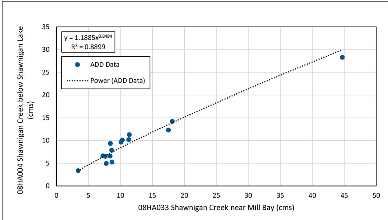
**Figure 10: Comparison of flood peak ADD data for Water Survey Canada gauges on Shawnigan Creek**
