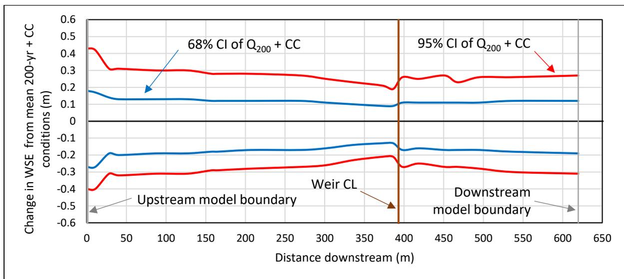
**Figure 20: Model sensitivity analysis results for change in Q200 plus CC flood flow for the closed Shawnigan Lake Weir scenario**
