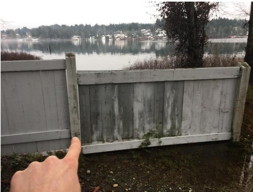
*Photo 5: Benchmark NHC 4496 (elevation= 117.356m), spike in fence post*
