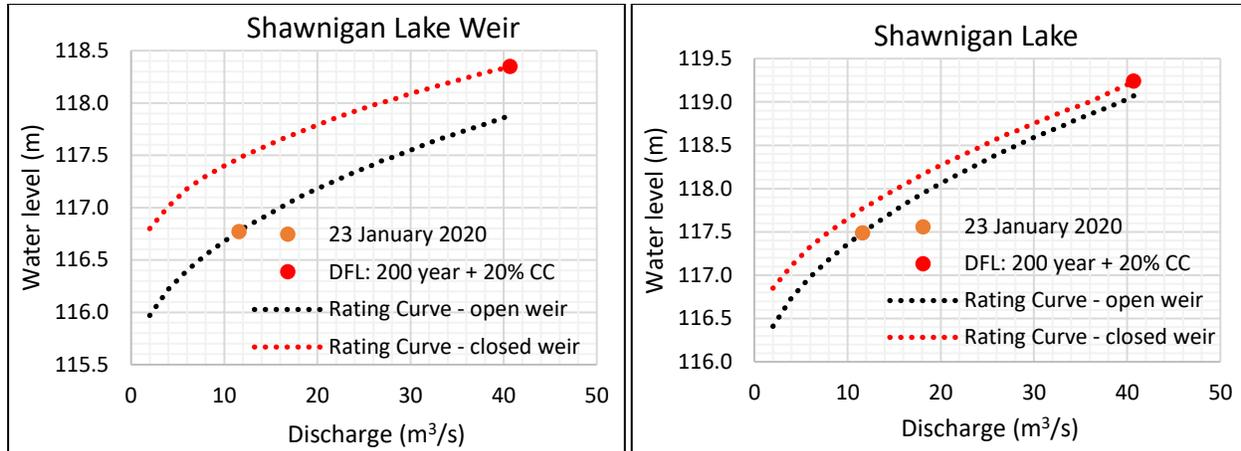
**Figure 19: Rating Curves for open and closed weir scenarios at Shawnigan Lake Weir (left) and Shawnigan Lake (right) using calibrated HEC-RAS model**
