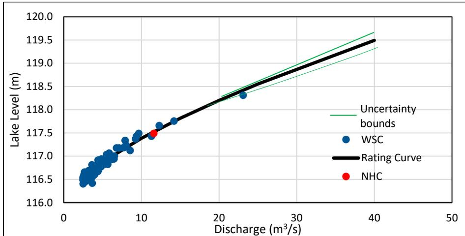
**Figure 11: Rating curve for the outlet of Shawnigan Lake as determined from coincident lake levels and discharges in Shawnigan Creek**
