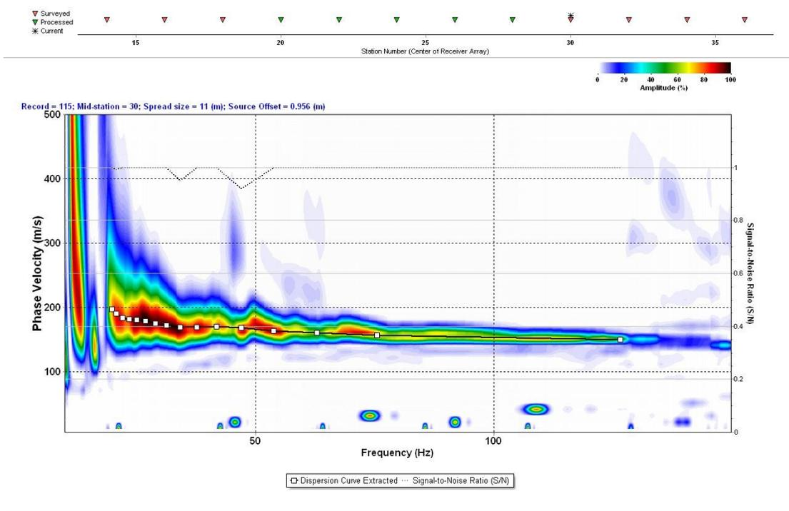
**MASW18-01:** Example time domain trace for active source (top) with resulting overtone image with picked dispersion curve (bottom).
