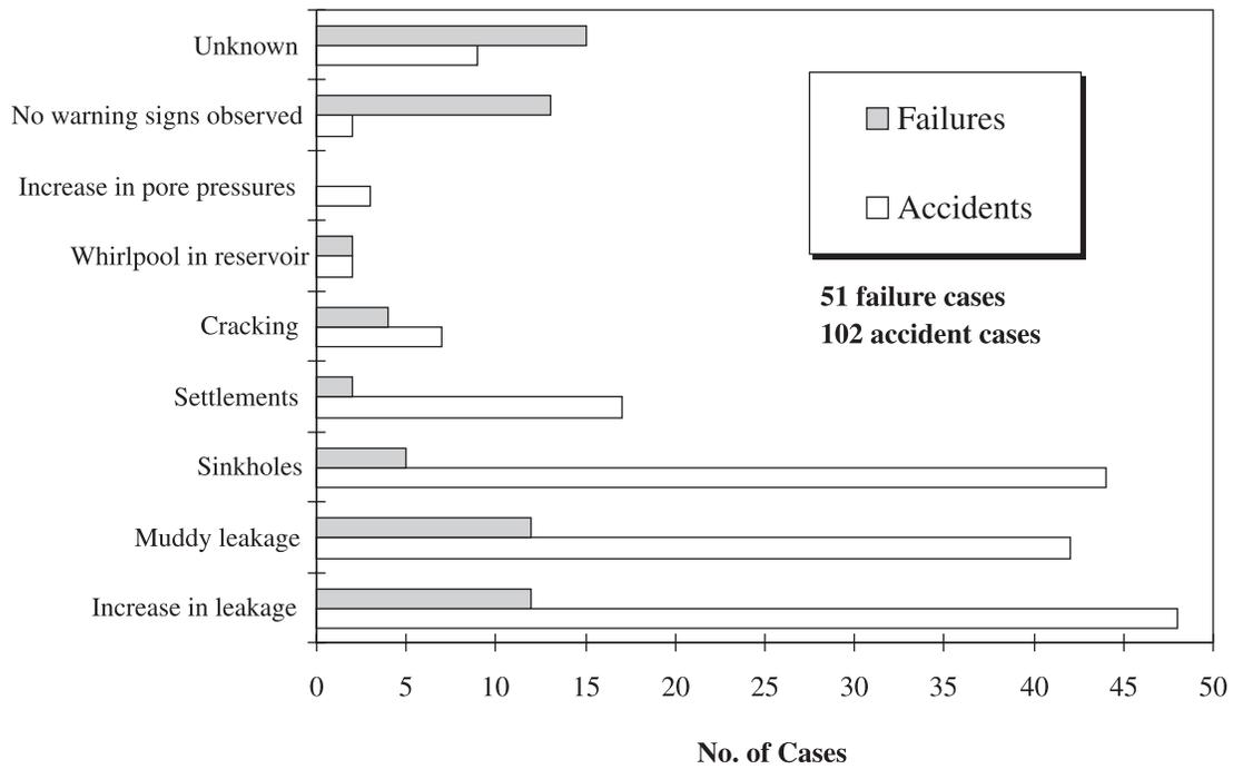
**Fig. 3.** Observations during piping incidents, with piping through the foundation.
