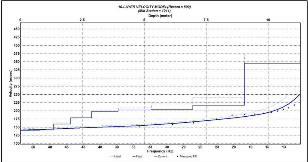
Figure MASW-3. 1D inversion result with fitted dispersion curve
