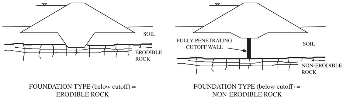
geology should be determined for both the soil and rock sections and the higher value obtained should be used, i.e.,  $w_{F(\text{fnd})}$  soil (type)  $\times w_{F(\text{cts})}$  (cutoff)  $\times w_{F(\text{sg})}$  (type), and  $w_{F(\text{fnd})}$  rock (type)  $\times w_{F(\text{ctr})}$  (cutoff)  $\times w_{F(\text{rg})}$  (type).
